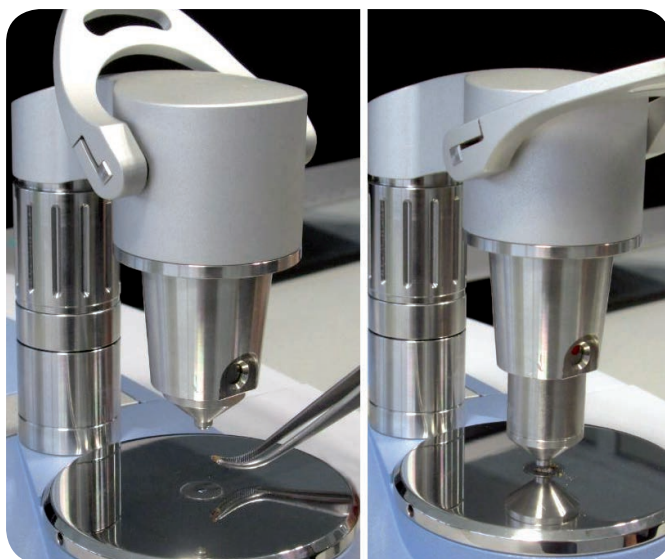
Figure 2: A kidney stone sample is being pressed on the diamond ATR crystal.
