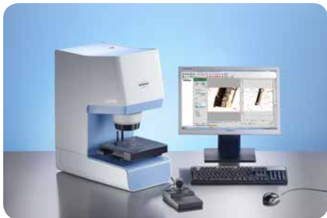
Figure 4: FTIR microscope LUMOS: Effective quality verification of coatings on smallest samples
