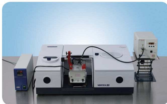
Figure 2: Bruker VERTEX 80 FTIR spectrometer with UV-irradiation source on the right side and heatable ATR accessory in the sample compartment.
